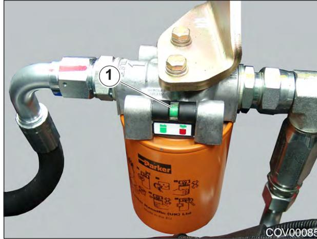
Figure 9.18 - Typical Hydraulic System Return Filter
