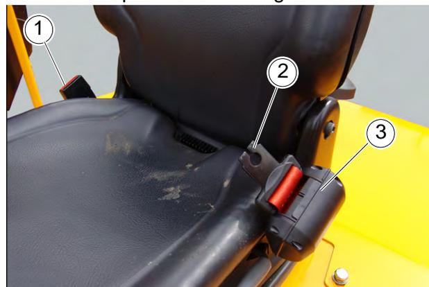
Figure 4.23 - Automatically Retracting Seat Belt
