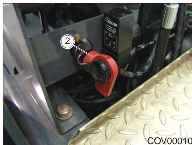
Figure 4.8 - Battery Isolator - OFF Position
