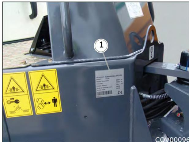
Figure 1.2 - Vehicle Identification Number Plate Location
